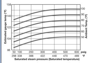
By knowing the saturated steam conditions and ambient temperature, the chart can estimate the gauge temperature, when the ABAC 's CV is used
