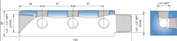
NOTE: 6 connections 1/4" NPT version are shown. In the 3 outlets version, the connection of one face are eliminated.
