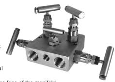
**Natural gas application:** The **M6GN** version has 3/8" orifice and soft seat. In this way it is possible to have bigger channels without diameter changes, to reduce pulsations in a gas line which may cause an error in the flow measurement as well as to assure a good drain where the wet gas and the hydrates are a problem.
